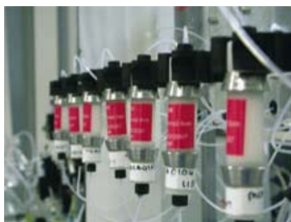
Photo 1: Array of Bioflash DFC cartridges in a BioSMB continuous downstream processing system
