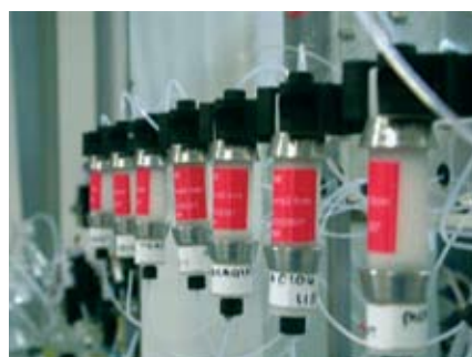
Photo 1: Array of Bioflash DFC cartridges in a BioSMB continuous downstream processing system
