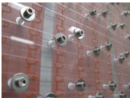
Fig. 2 Integrated 16 column position BioSMB™ valve cassette
