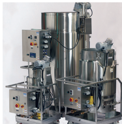
Photo 2: 50-L, 250-L, and 1,000-L S.U.B. single-use bioreactors from Thermo Fisher Scientific
